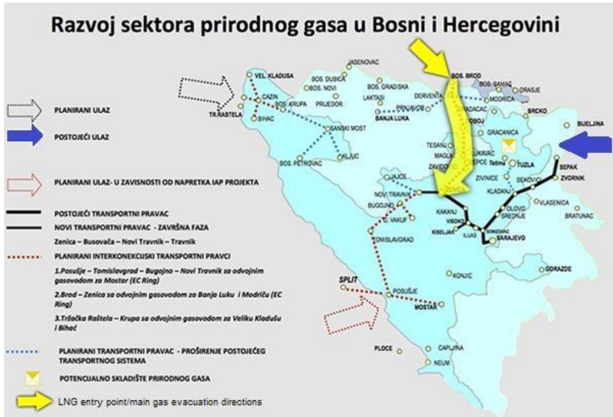
Fig. 2-4 Transport routes for gas from the LNG terminal on the island of Krk in the gas transmission system of Bosnia and Herzegovina (source: BH-Gas)
